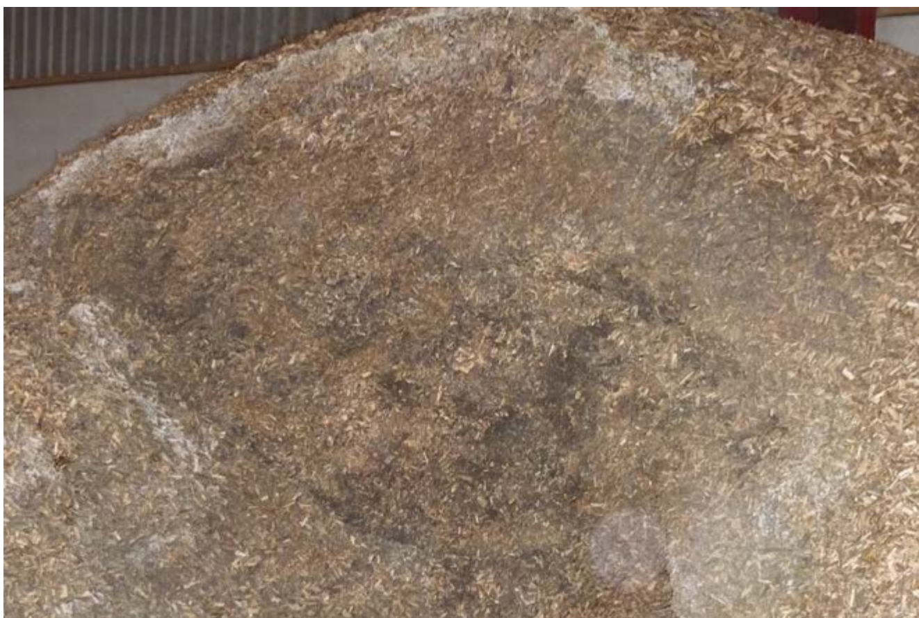
Figure 9. Microfungi in the centre of the indoor stack with cold air drying.
