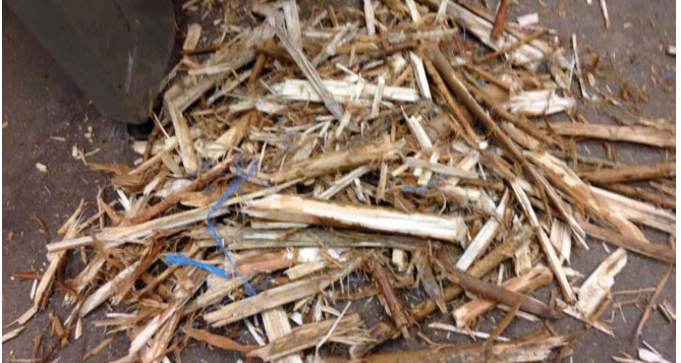
Figure 5. Blockage in the fuel feed owing to long fragments in the chips.
